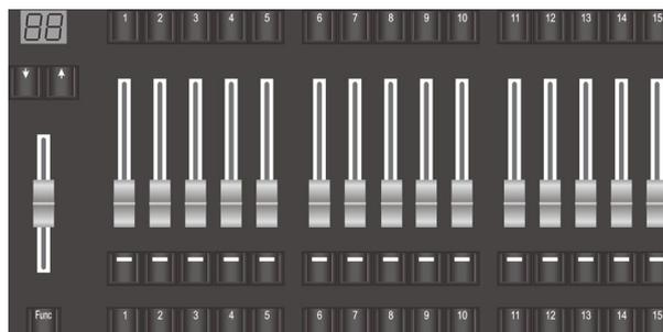
Pressing the **Func** key under the master fader can switch between the display of attribute setting and shortcut function to the display of the Fixed playback name.
