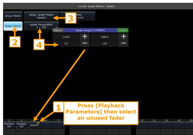
The Grand-Master fader can be set as the speed fader in the 'Manage Console' menu. However, the speed range of the speed source needs to be set by entering the 'Playback Parameters' menu of the playback fader.
