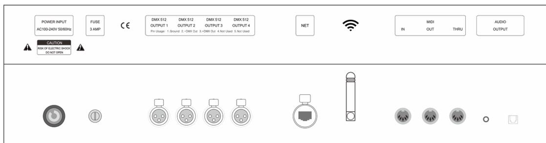
**Audio Output** --- one 3.5mm audio interface and one audio-optical interface allow you to connect with the audio device.
