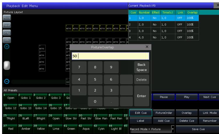
The running time will be divided equally for each fixture. That means if there are 5 fixtures run in 10s for the step. After setting the fixture overlap, each fixture uses 2s to finish its effect.
