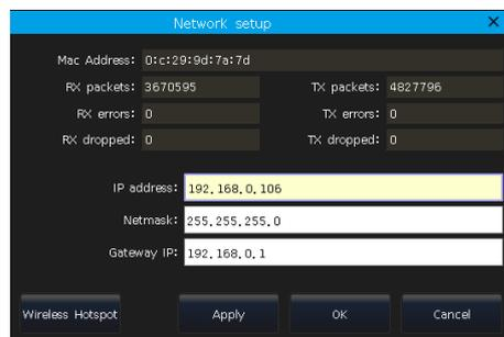
There is a **[Wireless Hotspot]** option allows you to open the WIFI function to connect with the App on remote devices. The SSID from the console is **'consoleWIFI'** and the WIFI password is **'87654321'**.
